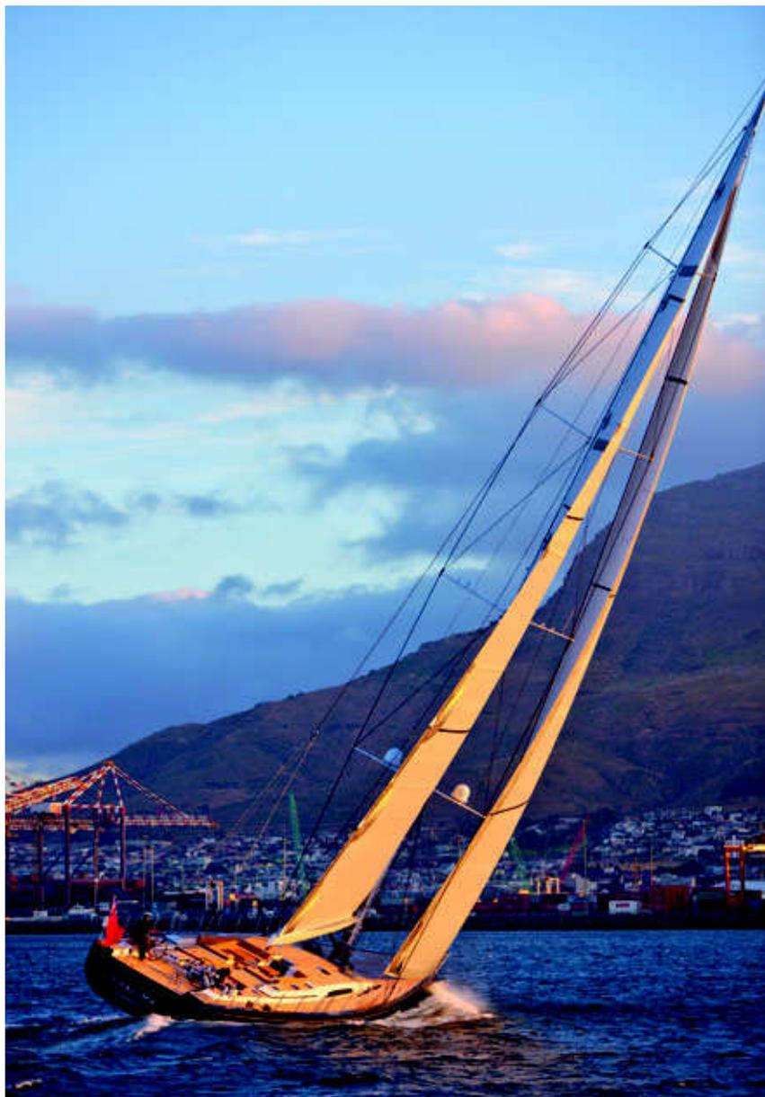
*Thalima* has a High Modulus carbon fibre mast and Park Avenue boom with Future Fibres PBO standing rigging.
