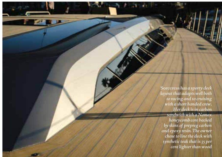
*Sorceress has a sporty deck layout that adapts well both to racing and to cruising with a short handed crew. Her deck is in carbon sandwich with a Nomex honeycomb core backed by skins of prepreg carbon and epoxy resin. The owner chose to line the deck with synthetic teak that is 35 per cent lighter than wood*
